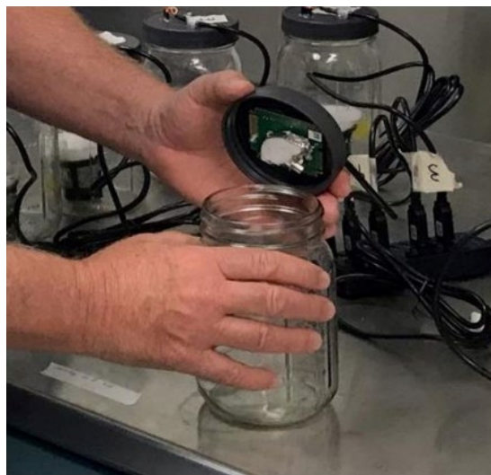
K30 CO 2 sensor affixed to the inner lid of a 950 mL jar with data acquisition via computer.
