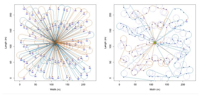
Fig. 2. Bale aggregation equipment simulation results: Left: Tractor, bales/trip = 1; Right: ABP, bales/trip = 8; simulation data: area = 5 ha; turning radius = 10 m; biomass yield/ha = 10 Mg; bale mass = 500 kg; harvester swath = 9 m; aspect ratio = 1.0; and random variation in biomass yield = 15 %.
