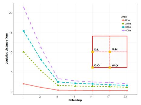
Fig. 4. Effect of number of bales/trip distance; insert – outlet locations: O:O -origin, W:O – along mid-width; O:L – along mid-length; M:M – field middle
