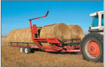
Fig. 1. An example of an automatic bale picker (ABP)
